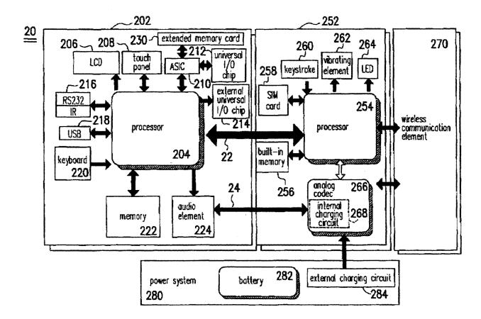
'219 patent, Figure 2. The '414 patent refers to the PDA 202 and wireless communication
