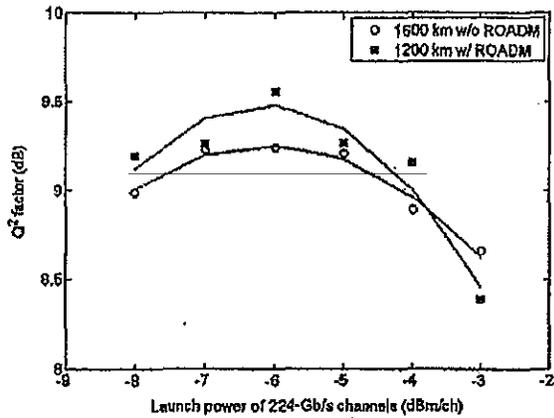
Fig. 8.  $Q^2$ -factor versus launch power of 224-Gb/s channels at 1200 km with ROADMs.
