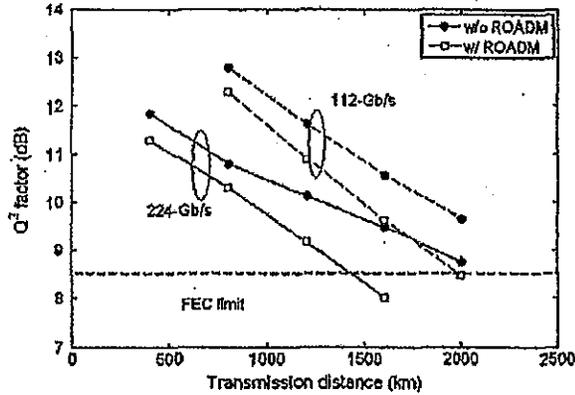
Fig. 9.  $Q^2$ -factor versus distance for 224-Gb/s and 112-Gb/s channels for the system with and without ROADMs.
