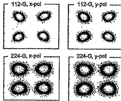
Fig. 6. Signal constellations of 112-Gb/s and 224-Gb/s CSRZ-PDM-QPSK at the input of the loop.
