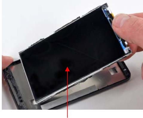
The HTC Evo includes an LCD video monitor that is attached to the wireless phone. The LCD video monitor displays video images processed by the Qualcomm processor (QSD8650).
