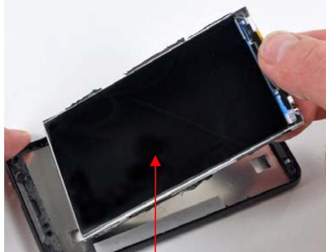
The HTC Evo includes an LCD video monitor that is attached to the wireless phone. The LCD video monitor displays video images processed by the Qualcomm processor (QSD8650).
