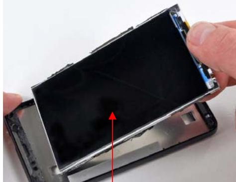
The HTC Evo includes an LCD video view screen that is attached to the PDA. The LCD video screen displays video images processed by the Qualcomm processor (QSD8650).
