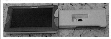
the magnifier having a second orientation wherein the handle and housing are angularly related, such that the handle can be positioned upon a surface and objects can be placed in front of the camera, The Aumed "Image" has a second orientation wherein the handle and housing are angularly related, such that the handle can be positioned upon a surface and objects can be placed in front of the camera, as shown in the image below from the Aumed flyer (Exhibit G):
