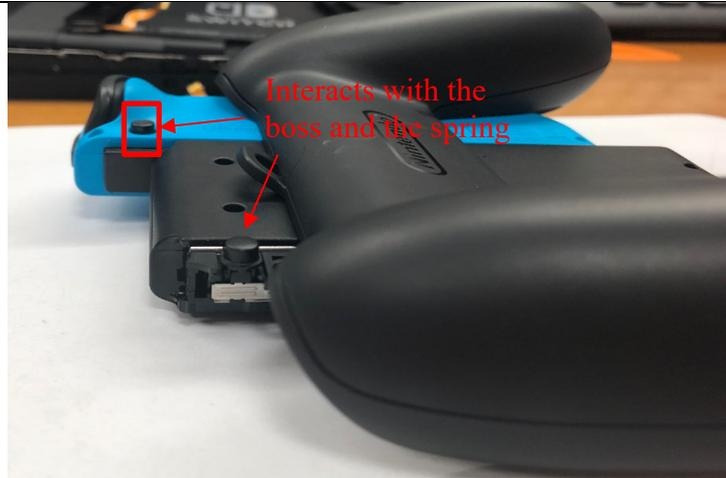
Structural bridge coupled with the electronic game control modules:
