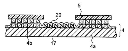
Figure 4C above represents the final product, with flexible substrates 5 connected to substrate 4 at terminal regions 4b via ACF 20. *Id.* at 10:15–25.
